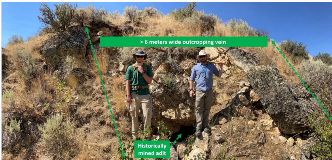
Figure 2 – Outcrop of greater than 6 meters wide vein with previously mined adit, over 650 meters from the main body of the 2020 resource estimate at Nutmeg Mountain. The vein is strongly banded and brecciated with near surface chalcedonic silica textures and cinnabar mineralization, indicating it is above the typical low-sulphidation epithermal gold-silver high-grade zone. To view image please click here
