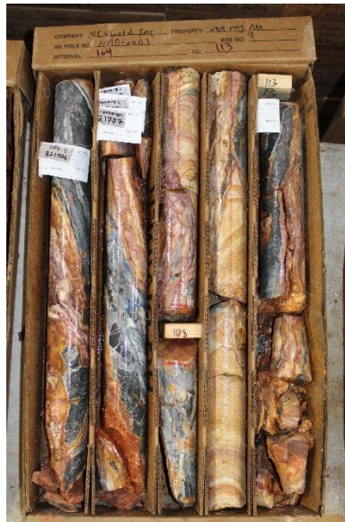
Figure 3 – Core Photos – NMD0003 from 31.7 meters to 34.4 meters (104 to 113 ft.), included in the zone that assayed 13.4 meters at 2.32 g/t Au. To view image please click here
