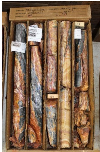
Figure 3 – Core Photos – NMD0003 from 31.7 meters to 34.4 meters (104 to 113 ft.), part of the zone that assayed 13.4 meters at 2.32 g/t Au. Released on April 13, 2023. To view image please click here
