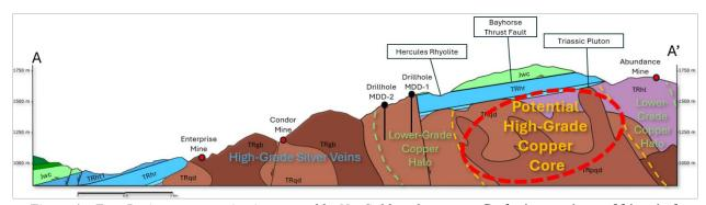
Figure 4 – Zeus Project cross-section interpreted by NevGold geology team. Geologic mapping and historical drilling at the Mineral Project (left and center of Figure) suggest a tilted porphyry deposit with the porphyry center east (right side of Figure) of the historical drillholes.
