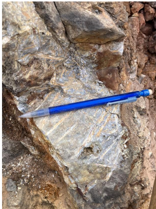
Figure 2 – Surface metallurgical grab sample from Resurrection Ridge: silicified and oxidized carbonate breccia with visible stibiconite (antimony) as elongated white crystals up to 6 cm long. To view image please click here
