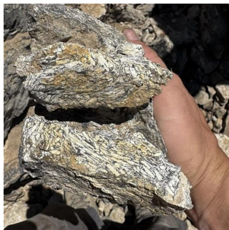
Figure 4 – Sample from road cut building new 2025 drill pads which assayed 6.8% antimony and 0.25 g/t Au in newly identified expansion part of the Project around the Bullet Zone discovery. Elongated white crystals are stibiconite ( Sb_3O_6(OH) ). To view image please click here
